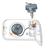
The filler cap is secured to the vehicle by a strap. For your convenience a holder is provided on the flap to store the cap whilst refuelling.
